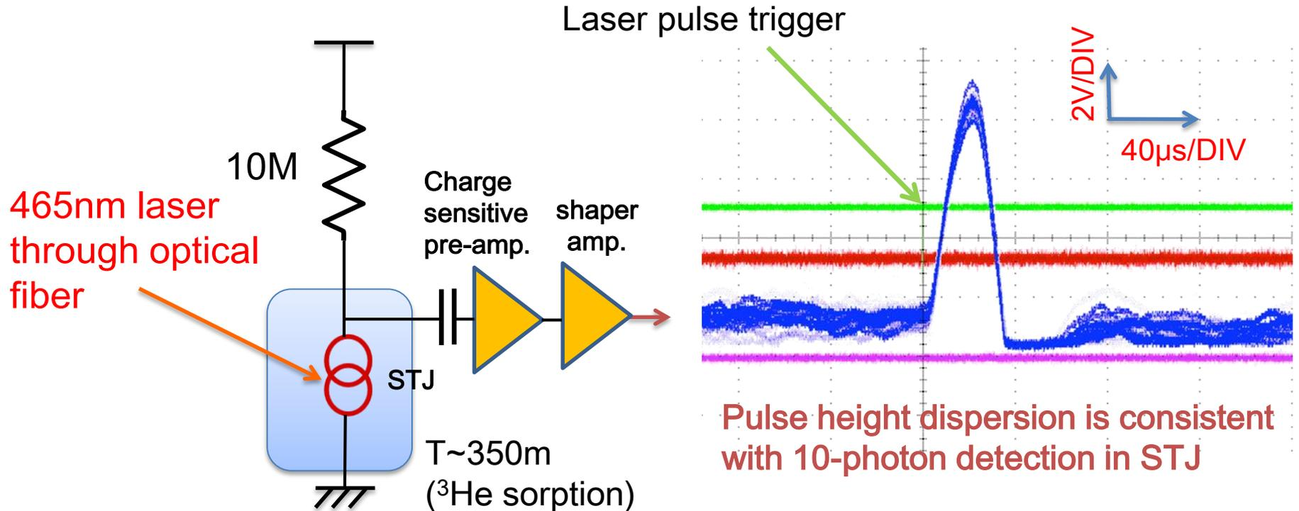
A response from Nb/Al-STJs to NIR-VIS photons at single-photon level was observed with a charge-sensitive amplifier at the room temperature
