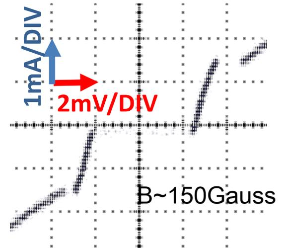
I-V curve of a STJ fabricated at KEK on a FD-SOI wafer
