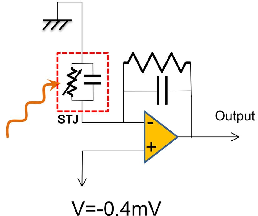
STJ readout circuit to apply a constant voltage on STJ as well as integrate the tunnel current from response to a photon.
