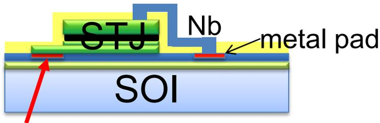
STJ lower layer has electrical contact with SOI circuit through **VIA**
