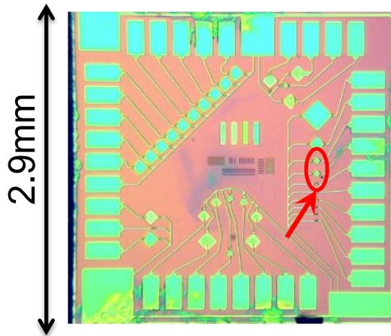
$50\mu\text{m} \times 50\mu\text{m}$  Nb/Al-STJ
