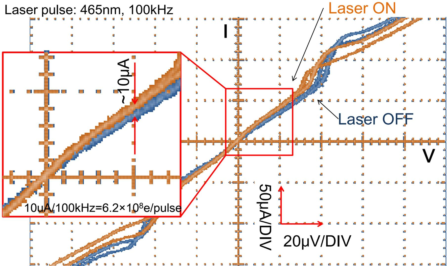
We observed an **increase of tunnel current** in Hf-STJ response to visible light
