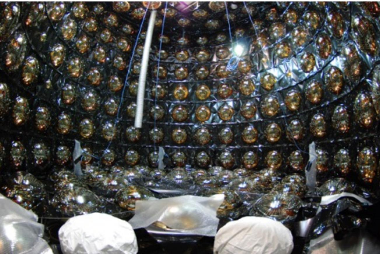
Inside of EGADS tank during PMT installation;
