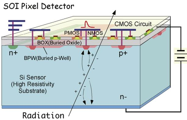
**Fig. 1.** Structure of the SOIPIX. The thickness of Si-sensor, BOX layer and CMOS circuit are 50–725  $\mu\text{m}$ , 0.20  $\mu\text{m}$  and 0.04  $\mu\text{m}$ , respectively.
