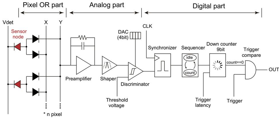
Fig. 4. PIXOR1 circuit for single channel. Analog and digital part are not mounted on sensor region (off-sensor).
