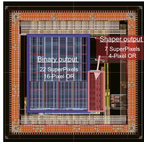
Fig. 5. Layout of the PIXOR1. The chip size is 6 mm  $\times$  6 mm.
