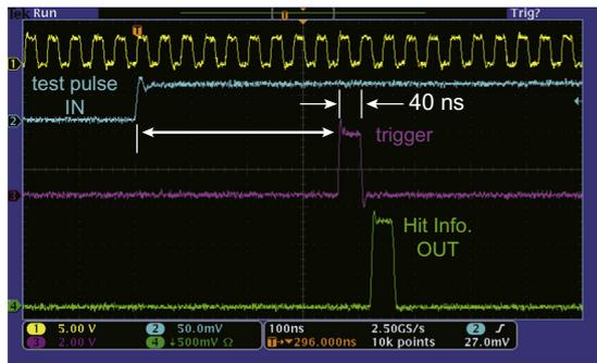
Fig. 8. Evaluation of trigger processing circuit. From top to bottom, clock (yellow), test pulse (cyan), trigger (magenta) and binary hit information (green). (For interpretation of the references to color in this figure caption, the reader is referred to the web version of this article.)
