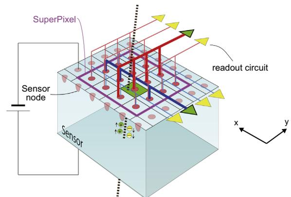
**Fig. 3.** Conceptual view of PIXOR (4  $\times$  4 Super Pixel case). A charged particle penetrates the green pixel. The signal is divided into X(blue)/Y(red) directions. In this figure, readout circuit is not shown. (For interpretation of the references to color in this figure caption, the reader is referred to the web version of this article.)
