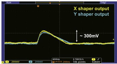
Fig. 7. Shaper output with a  $^{109}\text{Cd}$  X-ray source.
