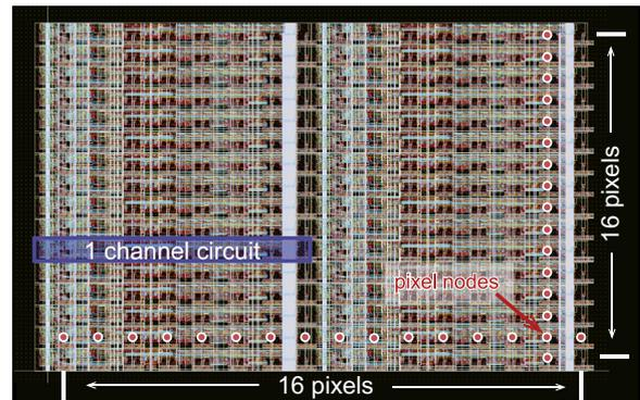
Fig. 6. Layout of a Super Pixel (16-pixel OR) which is the readout circuit on-sensor. In this paper, we report the result which is readout circuit off-sensor.
