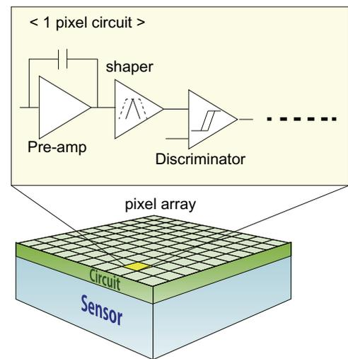
**Fig. 2.** Schematic view of chip-on-sensor. Each pixel has each readout circuit.
