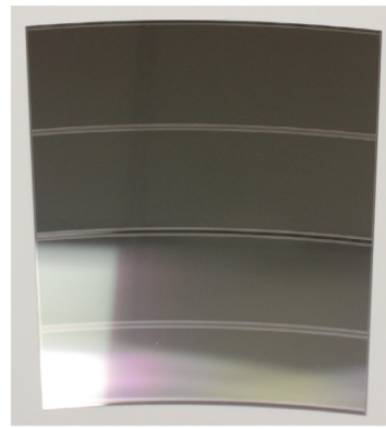
Fig. 1. The concept of the stereo annulus design is shown schematically in the left of this figure. A photograph of its first implementation in the ATLAS12EC is shown at right. Note that the schematic has the stereo angle skewed left while the ATLAS12EC has it skewed right.
