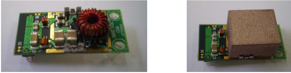
Figure 8. SM01C DC-DC converter without (left) and with (right) its polyethylene shielding box.
