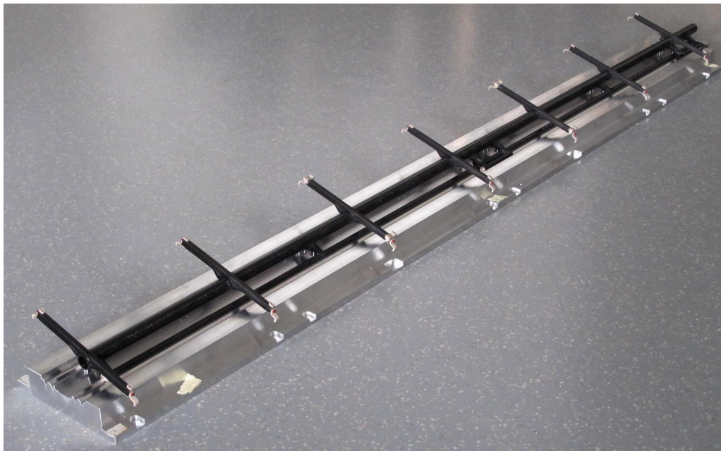
Figure 7. Photograph of the fully assembled CFRP backbone LS on its jig, before being equipped with the cooling plates, service bus and DSM modules.
