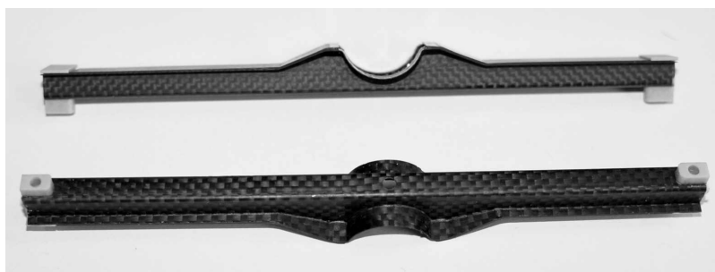
Figure 5. Upper and lower views of a prototype CFRP layup wing for the LS, including PEEK1000 attachments at the wing ends.
