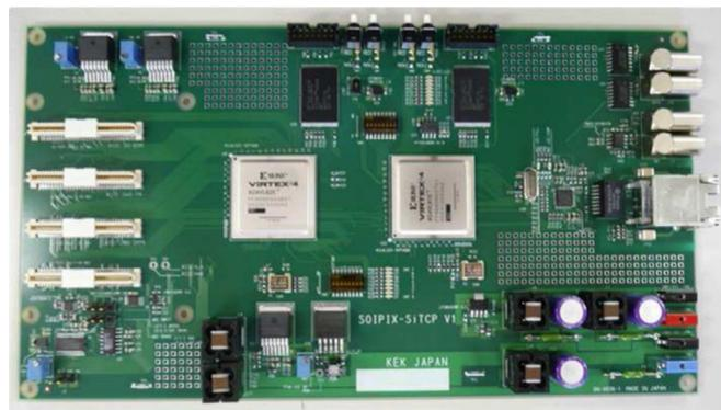
Fig. 3. Picture of the SEABAS board.
