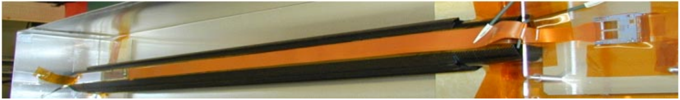
Fig. 3. Picture of the prototype test setup: two modules mounted on a CF structure
