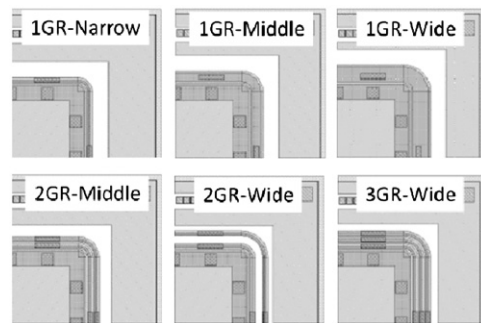
Fig. 7. Structure of multi guard ring.
