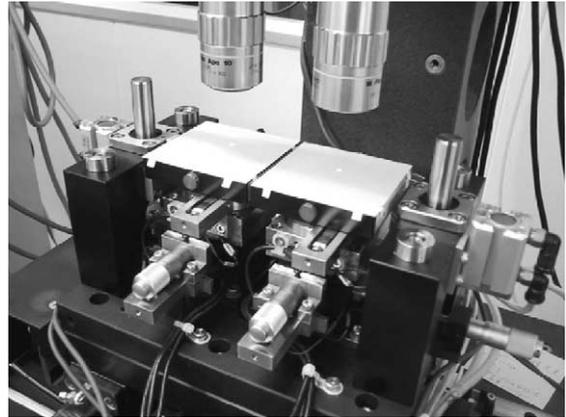
Fig. 8. Typical assembly microscope unit for sensor alignment.
