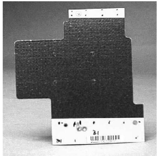
Fig. 5. Encapsulated VHCPG baseboard with BeO facing plates.
