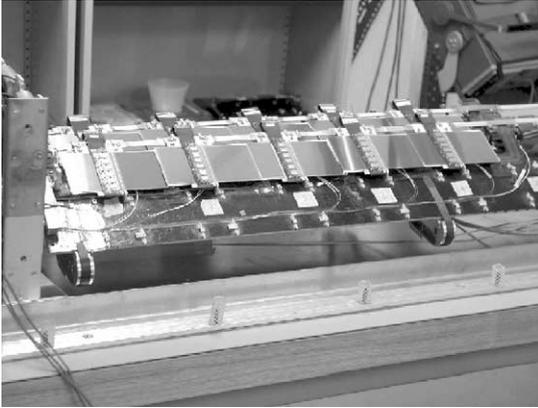
Fig. 18. Photograph of 10 barrel modules mounted on the carbon-fibre structure for system test.
