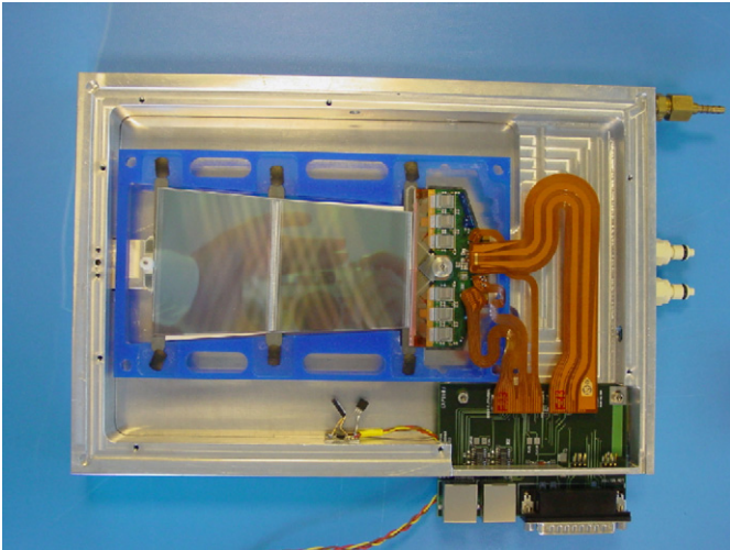
Fig. 30. Photo of an outer end-cap module supported by its transport frame inside its aluminium test box. The dry-air and coolant inlets are visible, as well as the support card.
