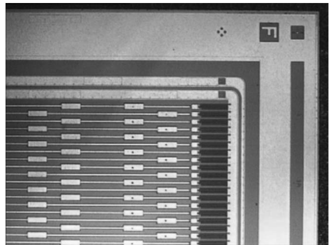
Fig. 7. Photograph of a corner of an SCT barrel silicon microstrip sensor supplied by Hamamatsu Photonics, showing the guard structure, a selection of fiducial alignment marks, the bias ring, polysilicon bias resistors and the metallisation above implant strips, including wire-bonding pads.
