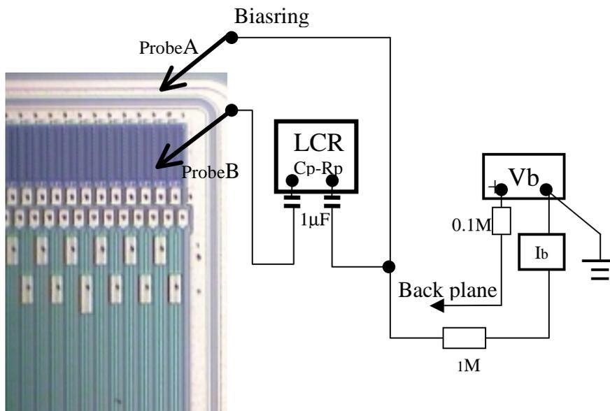
Figure 6: Setup for the polysilicon bias resistor measurement. A system based on external voltage source and ampere meter is an alternative, which can be configured from the interstrip resistance measurement setup (Fig. 8).
