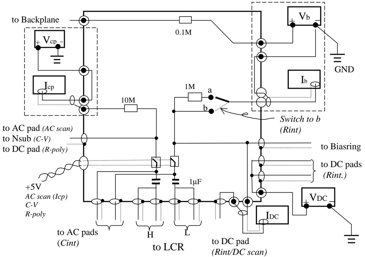
The probes are coaxial with the connections provided through Lemo connectors. The inputs to the LCR meter are switched, switching being controlled by a computer. Additional switch is used to by-pass  $1M\Omega$  resistor for interstrip resistance ( $R_{int}$ ) measurement. Two voltage and pico-ammeter systems can be replaced with source meters.
