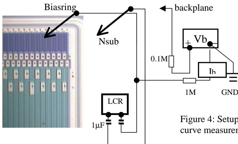
Figure 4: Setup for C-V curve measurement
