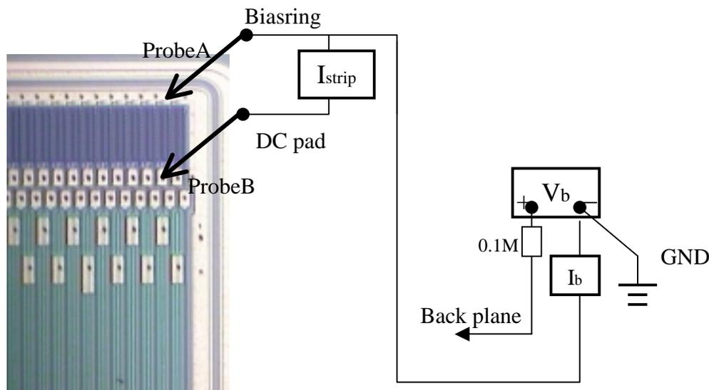
Figure 5: Setup for strip leak current measurement (DC scan).
