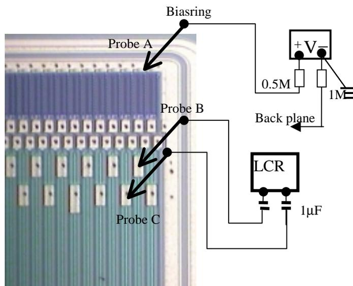
Figure 7: Setup for interstrip capacitance measurement.
