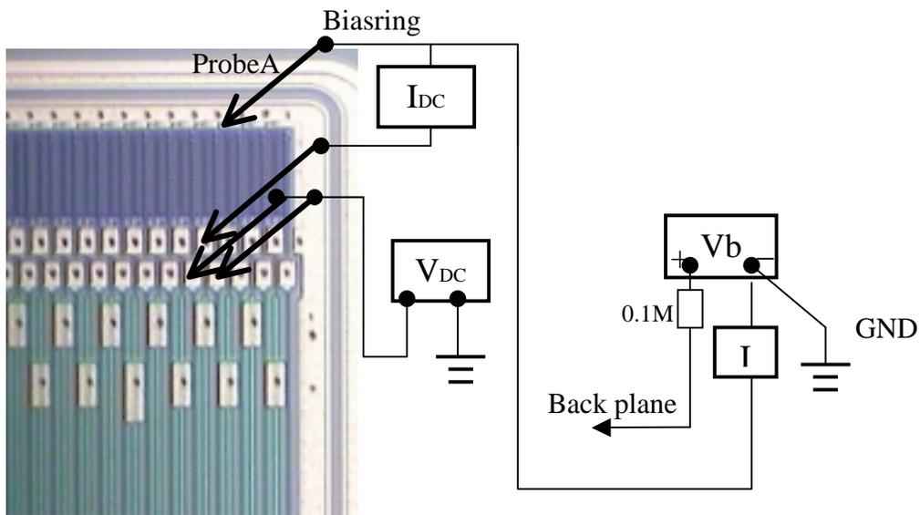
Figure 8: Setup for interstrip resistance measurement.
