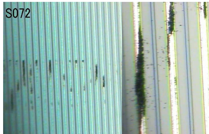
Fig. 8a Example of scratches observed for stereo sensors. (Right) Enlarged view.
