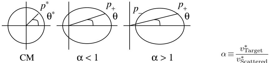
$$\frac{d\Omega}{d\Omega_{\pm}^*} = \pm \sqrt{D} \cos \theta \left( \frac{P^*}{P_{\pm}} \right)^2 \quad D \equiv 1 + \gamma^2 (1 - \alpha^2) \tan^2 \theta$$
