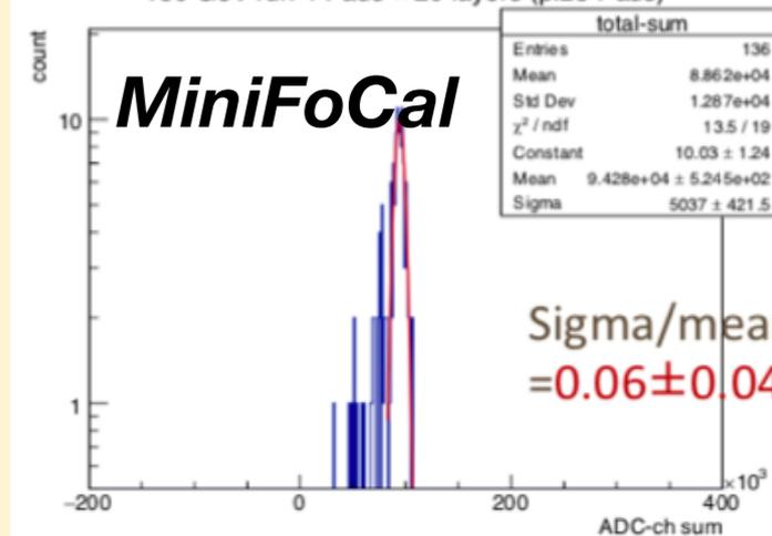
Initial analysis shows the resolution of the detector to be around 6% (work in progress)
