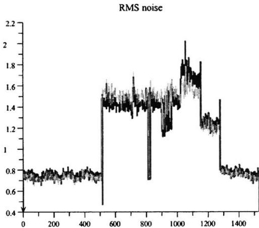
Fig. 5. Noise (dark) and Dnoise (light) on a stave. Channels 1–512 and 1350–1536 are unbonded, channels 513–1290 are bonded to two sensors (full load). Channels 1050–1290 are damaged, resulting in excess leakage current and noise. Channels 1291–1349 are bonded to one sensor. Two-sensor noise is about 1200 electrons.
