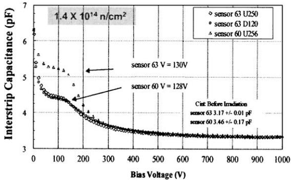
Fig. 8. Interstrip capacitance of two irradiated sensors: one pair and two pairs for each.
