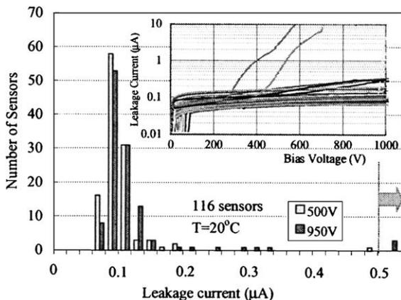
Fig. 7. Leakage current distributions of 116 prototype sensors at 500 and 950 V. The overflows are histogrammed on the extreme right. The inset shows the  $I$ - $V$  curves of all the sensors.
