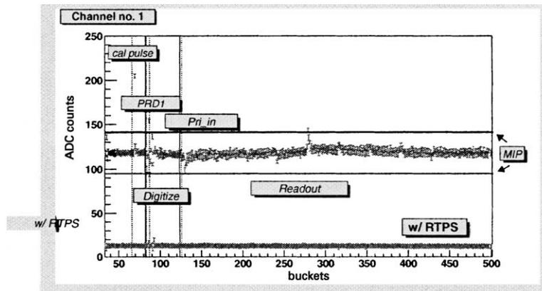
Fig. 6. Study of dead-timeless operation with RTPS off (top) and on (bottom) curves. Various operating conditions of the SVX4 chip are indicated.
