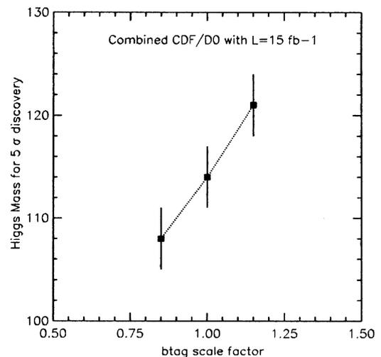
Fig. 1. Higgs mass reach for a  $5\sigma$  discovery as a function of the b-tag efficiency relative to a nominal value of 65% for an integrated luminosity of  $15\text{fb}^{-1}$  per experiment.
