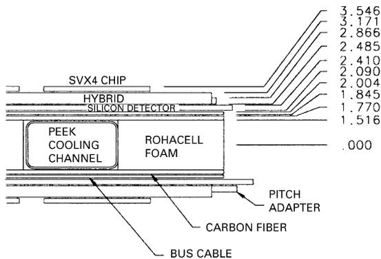
Fig. 4. Detailed view of one-half of the end of the stave showing mechanical and cooling features.
